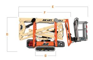
Platform Width 30-in / .76-m Platform Length 52-in / 1.34-m Machine Width 29-in / 75-cm Machine Height 6-ft 6-in / 1.98-m Machine Length 13-ft 2-in / 4.02-m Machine Length Without Platform 11-ft 2-in / 3.40-m Track length 4-ft 1-in / 1.24-m Outrigger Footprint Length 9-ft 8-in / 3.0-m Outrigger Footprint Width 9-ft 8-in / 3.0-m J. Outrigger Pad Diameter 11.8-in / 30-cm
